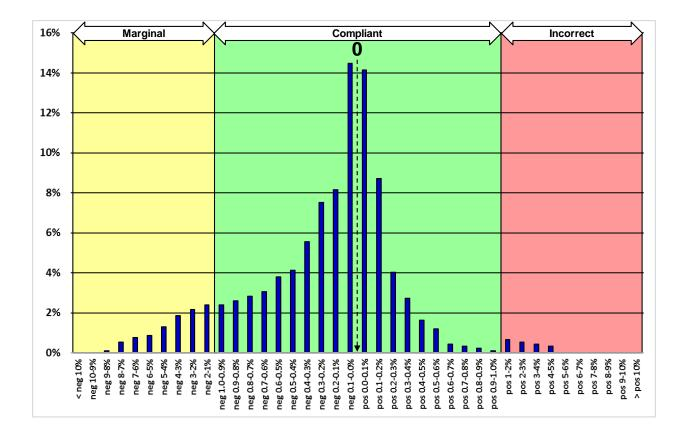
Adding the bucket percentages (blue bars) in the green range shows that 88% of the samples are within spec. The sum for bars in the yellow range is 10%, while the bars in the red range add up to 2%, accounting for 100% of the samples. Applying the above Apdex formula to the number of samples shown in this distribution chart yields: Apdex = 0.88 + 0.10/2 = 0.93. The distribution has an Apdex score of 0.93 [+/-1%], which has a rating of Good.
