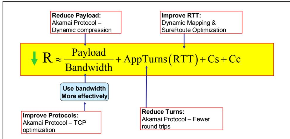
Figure 2 – Acceleration “Levers” Akamai Uses to Improve SAP Performance
