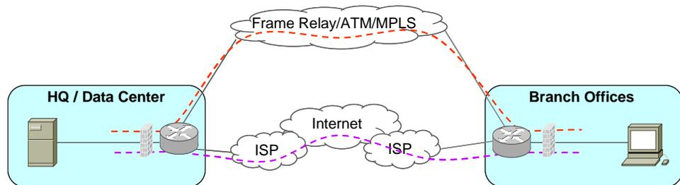
**Figure 1 - Providing a second link to the branch office**
