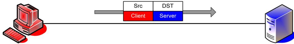
**Figure 3 - Source / Destination Addressing, No Acceleration Appliances**
