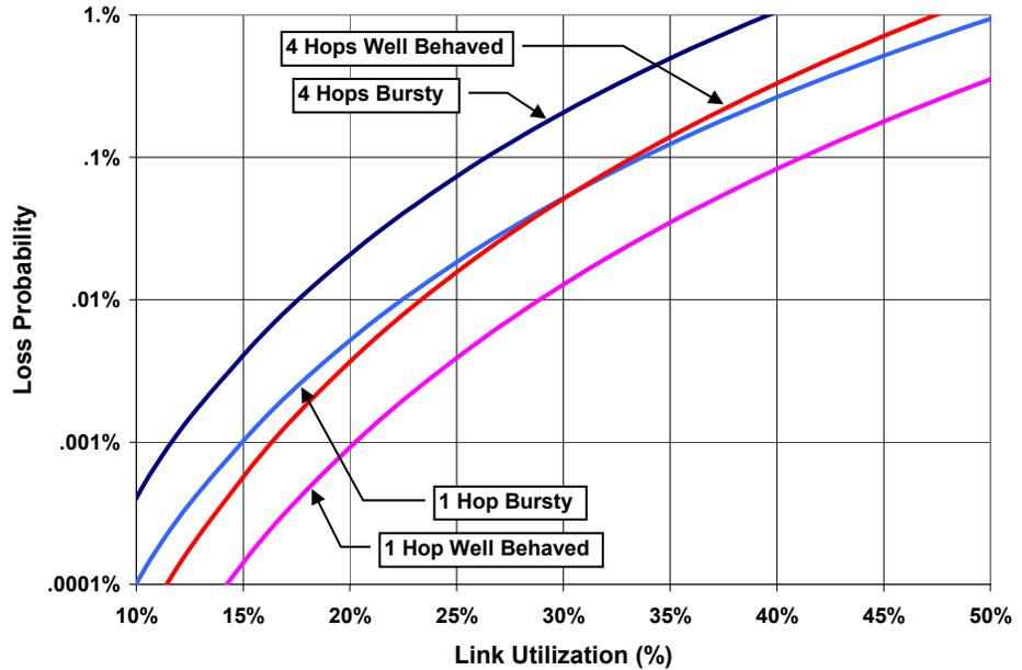
**Figure 1 - Effect of Link Utilization on Packet Loss Probability**
