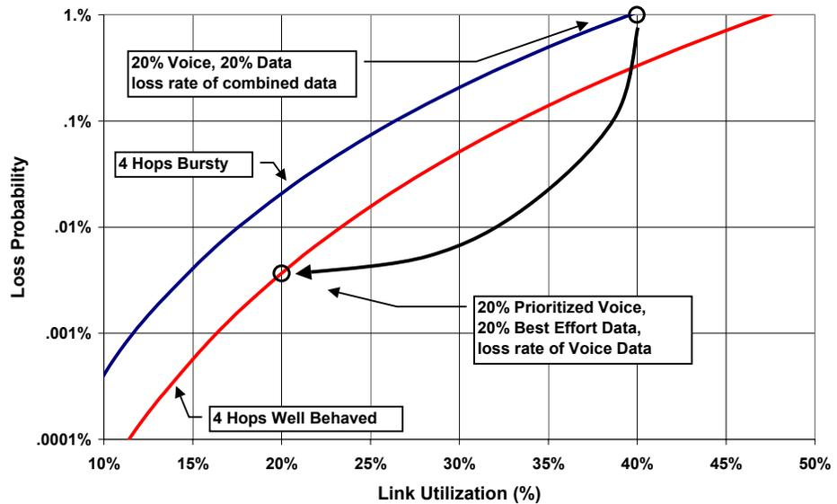
Figure 3 - Effect of Adding QoS on Voice/Video Packet Loss
