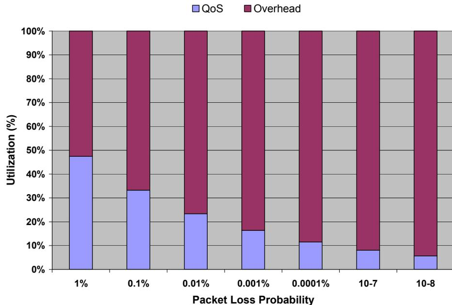
**Figure 4 - Overhead Required for 4-Hop Network Connection Using QoS**
