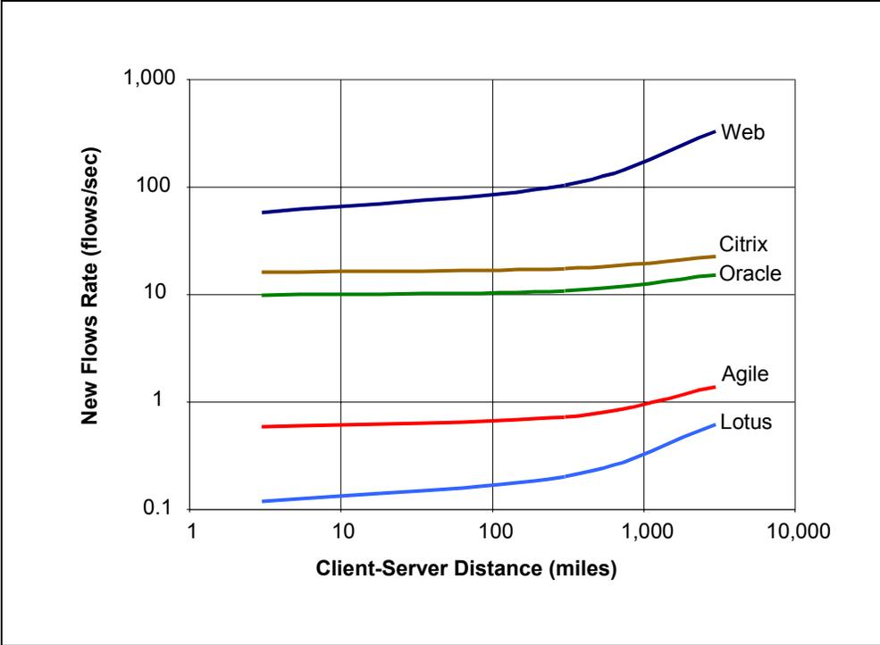
Figure 5 – Estimated Flow Rates for Active Users Filling an OC3 Circuit
