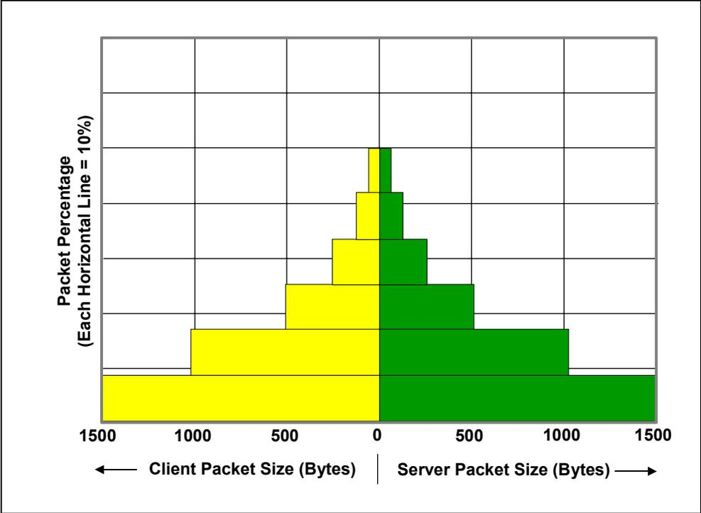
Figure 2 – Progressive Doubling PMC
